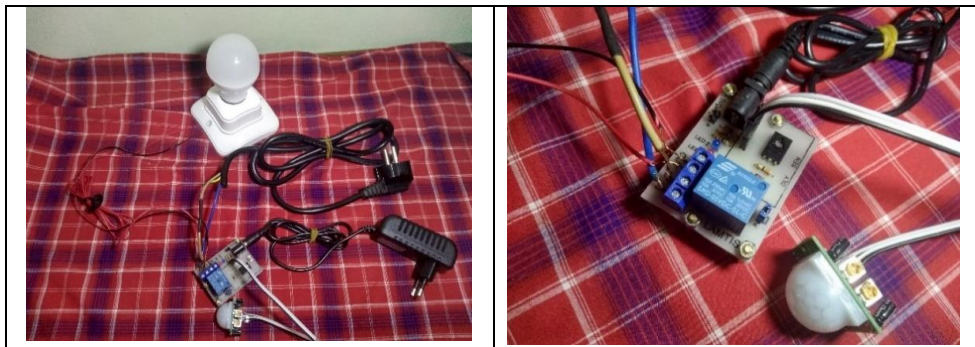
Fig 4. The circuit of the motion sensor light system and the circuit on the relay module.
