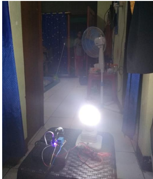
Fig 8. Sensor detects motion at a distance of 5 meters.
