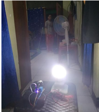
Fig 7. Sensor detects motion at a distance of 4 meters.
