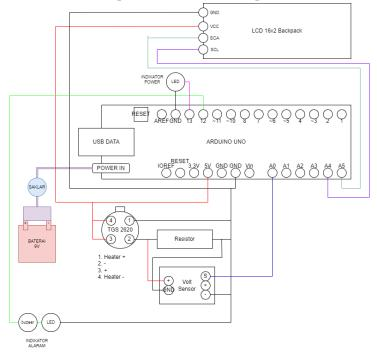
Fig 1. The diagram design of the system
