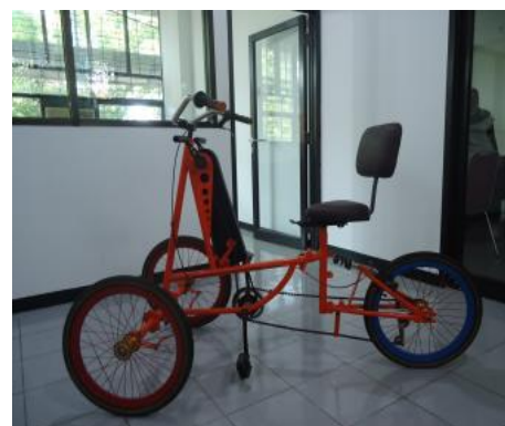
Fig 4. Post-stroke bicycle Re-design [2]
