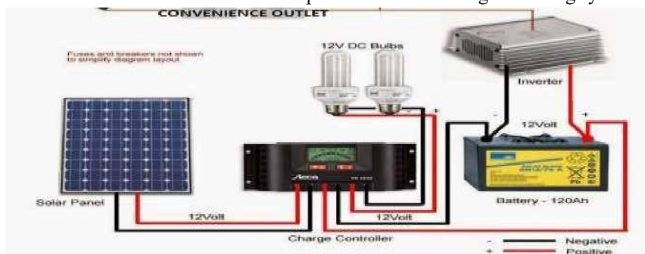
Fig 7. Schematic Diagram of the Solar Charging Station Wiring Diagram Sunlight Tracking System
