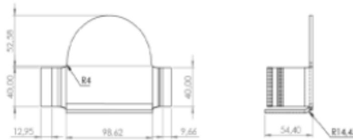
Fig 3. Rear Axle Bumper Bracket RH Lower Part (mm)
