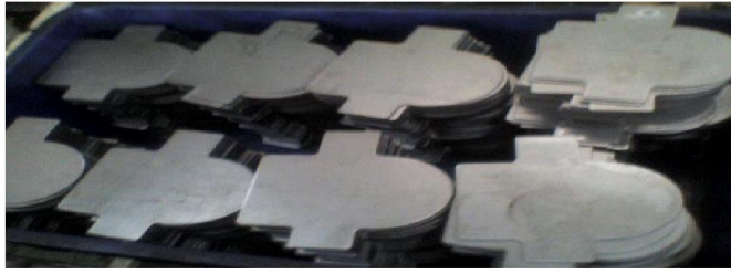
Fig 7. Result of Blanking Bracket Bumper Rear Axle RH Lower Part
