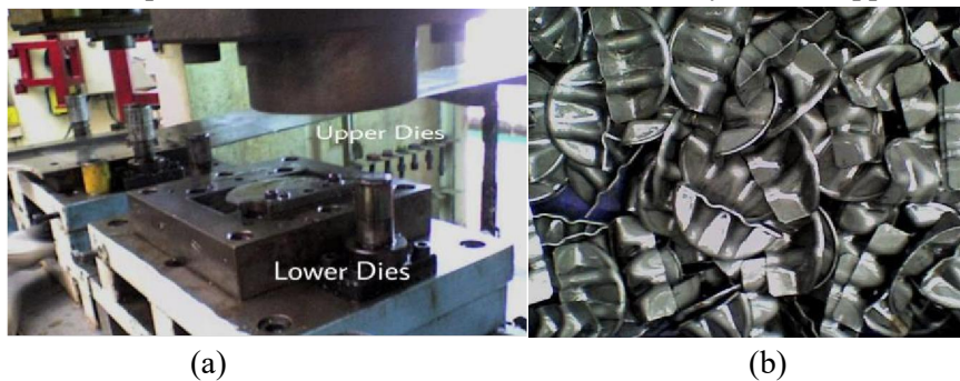
Fig 9. (a) Drawing Dies Bumper Bracket RH Rear Axle Upper Part, (b) Results Bracket Drawing Bumper RH Rear Axle Upper Part
