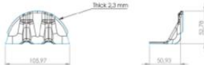
Fig 4. Rear Axle Bumper Bracket RH Upper Part (mm)
