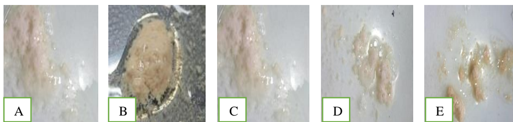
Fig. 5. The characteristics of the curd produced in depositional optimization ammonium sulfate (A) 40% with compactness level curd (low: +) , (B) 45% (moderate: ++), (C) 50% (low: +), (D) 55% (low: +) and (E) 60% (low: +)
